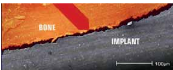
Control – Overload testing results in fracture at the interface.
